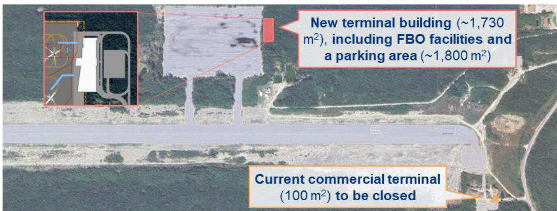
Figure 43. Passenger terminal development (1/2)
